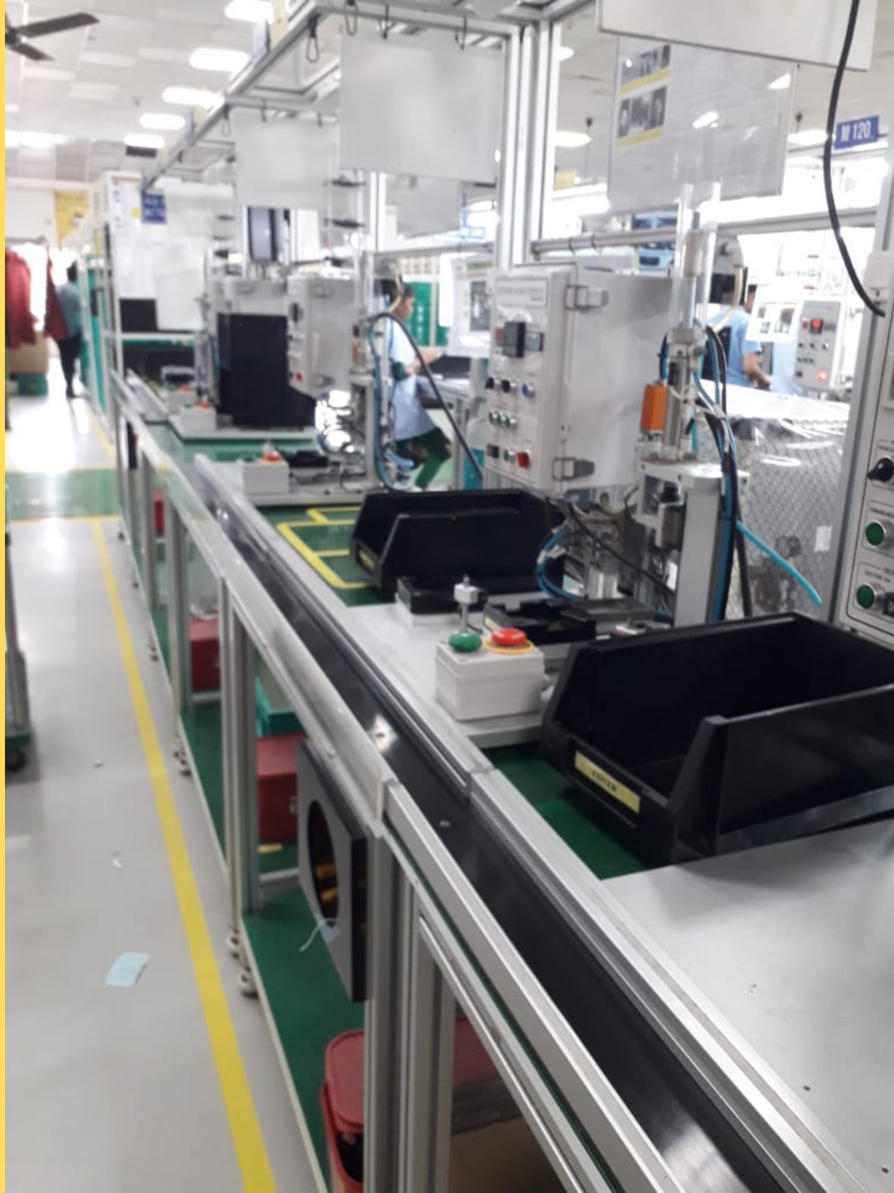
Electronic Module - Transfer unit for Food product packing machine
